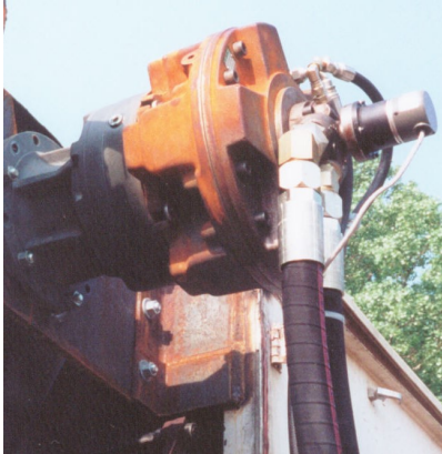
SAI Motor, Gear Box and Encoder
